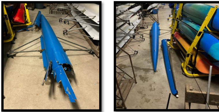
Figure 2. Photos of Rowing Scull (post collision) at Baltimore Community Rowing Facility. 07August 2024 Taken by Coast Guard Investigator.
