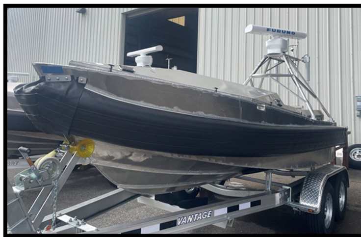
Figure 1. Photograph of an unmanned Global Autonomous Reconnaissance Craft, trailered. This is not the photo of the VICAR 602 but of a similar hull and design. Obtained from Internet.
