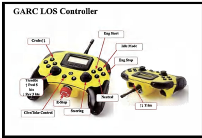
Figure 10. GARC Controller Configuration. Obtained from MAPC.
